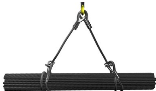
Double Wrap Choker Hitch
