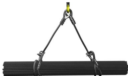
Double Wrap Choker Hitch
